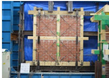
Fig. 1 – Timber frame with masonry infill (S2)
