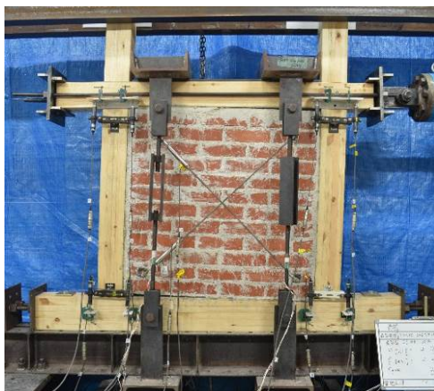
Fig. 5 – Deformation of the specimens at 0.03 rad
