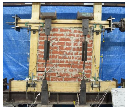
Fig. 5 – Deformation of the specimens at 0.03 rad
