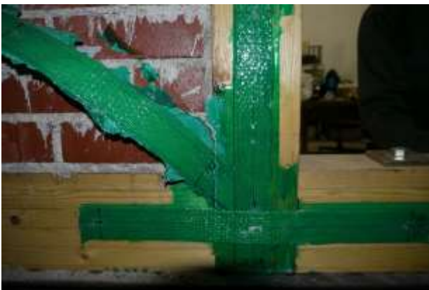
Figure 13: Fracture of the AFRP sheet on the back side of the bottom connection (TFM-CH-AFRP)
