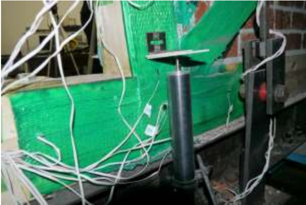
Figure 18: Fracture of the AFRP sheet on the back side of the bottom right connection (S5)
