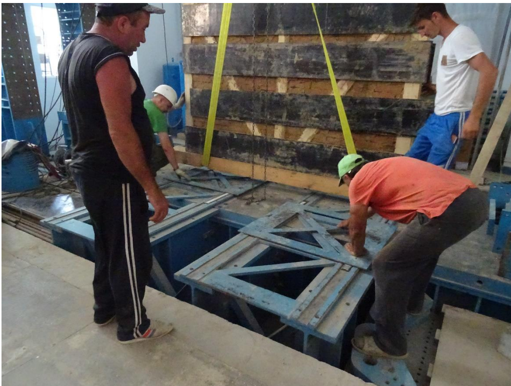
11. The metal plates on which the specimen is slid are removed, together with the rollers and the other metal plates with edges for rollers
