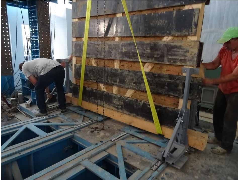
11. The metal plates on which the specimen is slid are removed, together with the rollers and the other metal plates with edges for rollers
