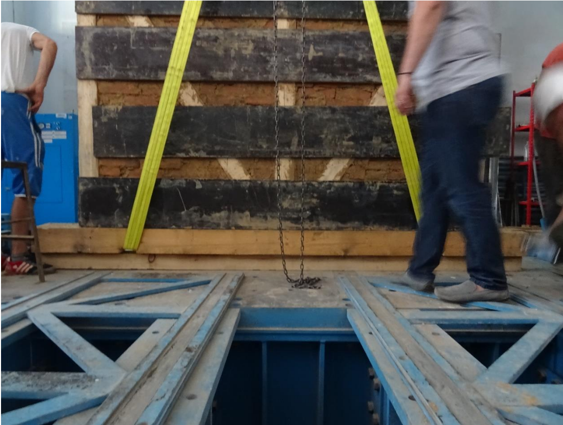
13. The specimen is centered at the bottom and fixed by bolts to the reaction slab (30 min)
