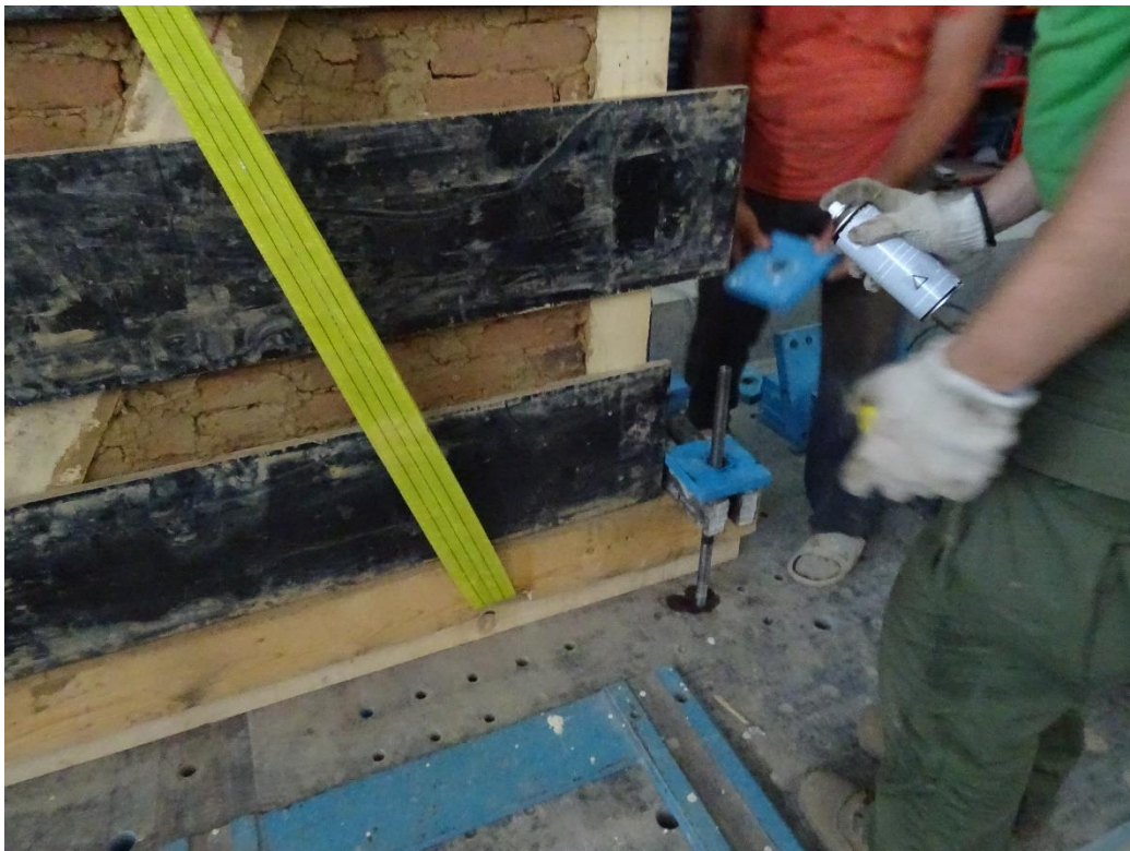
14. The specimen is fixed in horizontal direction at the bottom, with bolts and stoppers and the horizontal bolts to be pushed until needed (15 min)
