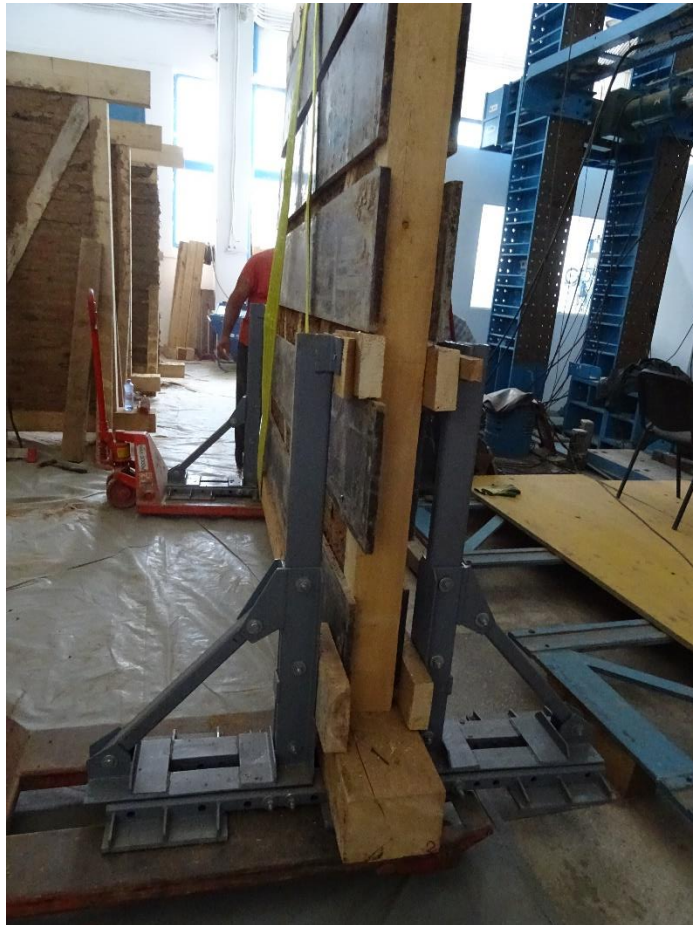
6. The specimen is fixed in the steel supports by wedges and screw nails
